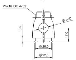
for holding rods with Ø12 mm
