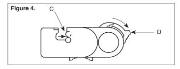
3. Insert cable into the tool, making sure that the cable does not touch the cutters. Advance the pressure rollers by means of the cam wheel until the cable is just touching the 'V' of the cutter cassette, and set the maximum position of the cam wheel by means of the slide, see figure 7 by moving it backwards towards the cam wheel. The cable should be free to rotate showing no signs of friction.
