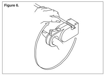
5. To remove the stripped cable, retract the pressure rollers by using the cam wheel, and remove the stripped pieces of insulating and braid materials from the cable and check that all cuts are of the required depth.
