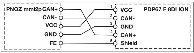
Connection to a decentralised input module PDP67
