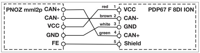
Connection when using the PSS SB BUSCABLE LC in conjunction with a Pilz self-assembly "PSS67 M12 connector" (see order reference in the Technical Catalogue)
