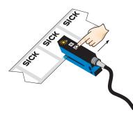
Press both the "+" and "-" buttons together, hold > 1 s and than release the teach-in buttons. The red LED flashes.
