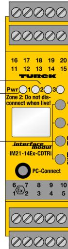
The rotation speed monitor IM21-14EX-CDTRI monitors frequencies, rotation speeds and pulse trains of rotating motor, gear or turbine parts according to over or undershoot of adjusted limit values. A display at the front indicates the current value.
