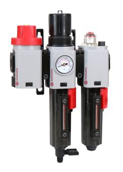
**Diaphragm Type:** Relieving Drain: Manual or automatic Automatic drain operating conditions (float operated): Bowl pressure required to close drain: > 0.35 bar (5 psi) Bowl pressure required to open drain: ≤ 0.2 bar (2.9 psi) Minimum air flow required to close drain: 1 dm<sup>3</sup>/s.
