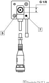
1 Switch OUT 1, green LED 2 Switch OUT 2, red LED 3 Dustproof protector 4 Connector M12 x 1 5 Inlet port Alternative inlet port G1/8 plugged
