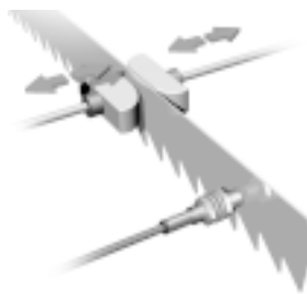
Measuring deflection of a saw blade. The saw blade position is detected by the sensor and the blade guide mechanism accordingly adjusted.
