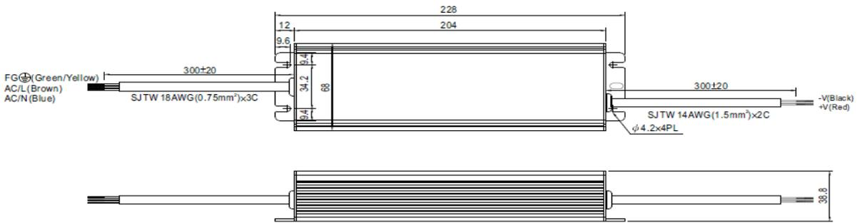
※IP67 rated. Cable for I/O connection.
