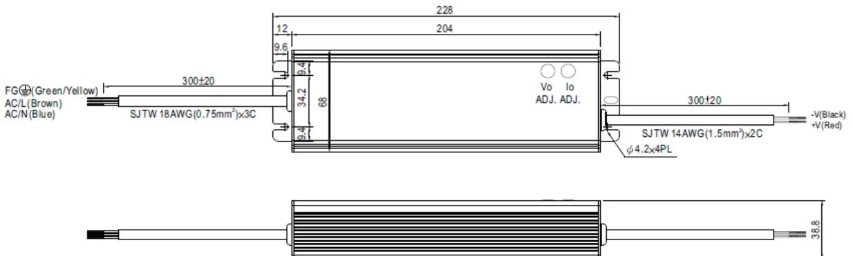
※ IP65 rated. Output voltage and constant current level can be adjusted through internal potential meter.
