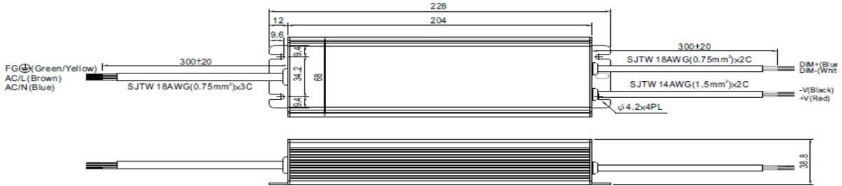
※ IP67 rated. Output constant current level can be adjusted through output cable by connecting a resistor or 1 ~ 10V dc or 10V PWM signal between DIM+ and DIM-.
