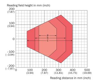
For devices with plastic reading window, the depth of field is reduced by approx. 10 %.
