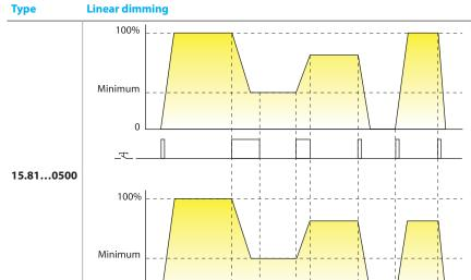
**Operating mode without memory:** at switch-off, the light level is not memorized.
