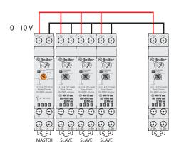
This new system is modular, adaptable to every need and allows control of multiple lamps through a single control device called the "Master Dimmer" Type 15.10.8.230.0010.
