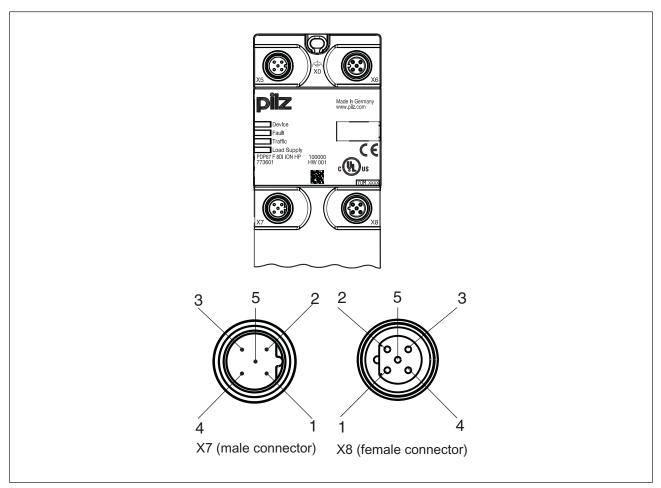
Fig.: Pin assignment for the supply voltage
