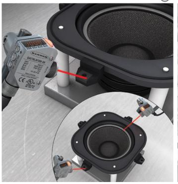
The Q4X verifies presence of a single spacer while also monitoring intensity to verify adhesive side is down. Master/slave mode provides cross talk avoidance when using multiple sensors in close proximity.
