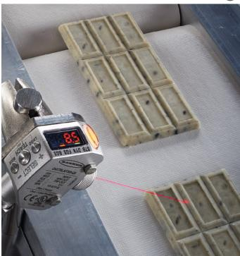
The Q4X detects the small change in height on multicolored candy bars. The display, with decimal point, can show distance from the sensor or relative to the conveyor.
