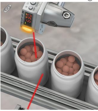
The Q4X analog sensor uses its averaging trigger mode to provide a more consistent fill level measurement across inconsistent surfaces, such as pills inside a bottle.
