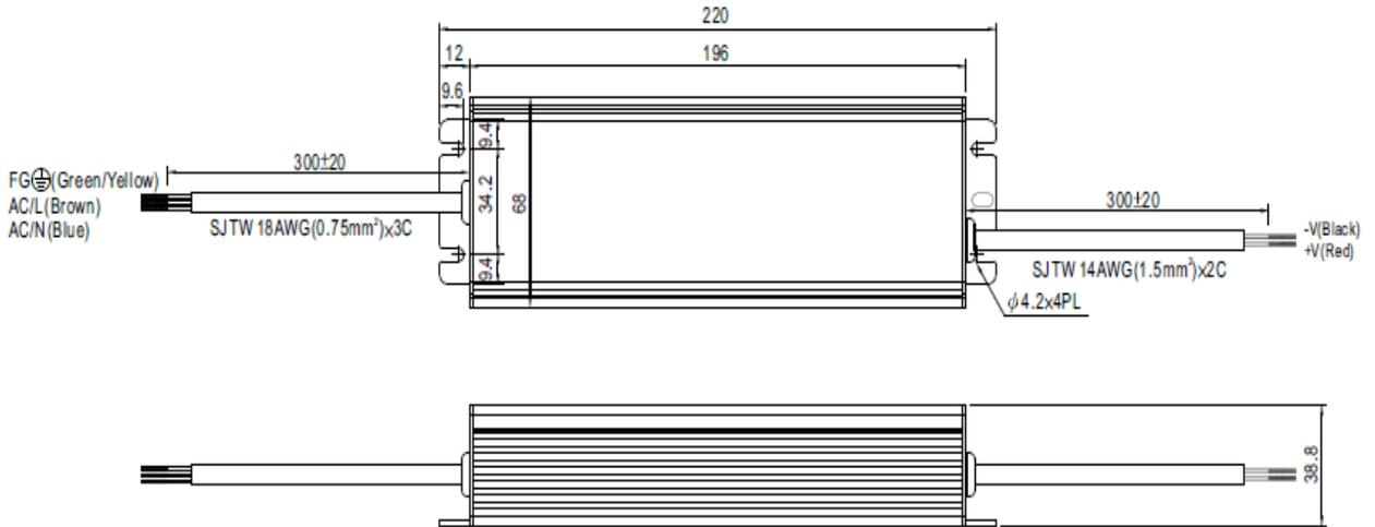
※IP67 rated. Cable for I/O connection.
