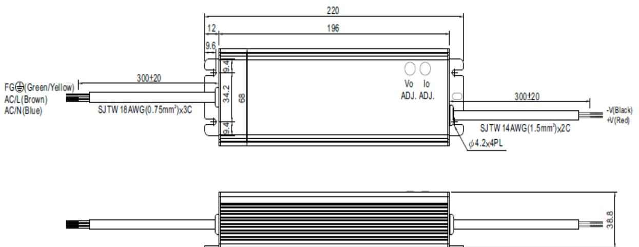
※ IP65 rated. Output voltage and constant current level can be adjusted through internal potential meter.
