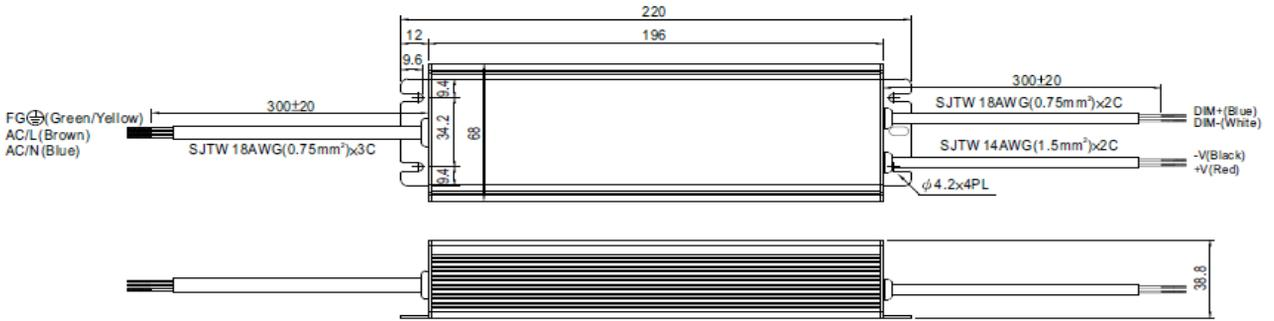
※ IP67 rated. Output constant current level can be adjusted through output cable by connecting a resistor or 1 ~ 10Vdc or 10V PWM signal between DIM+ and DIM-.
