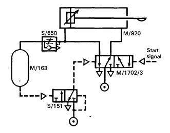
The circuit illustrated above is a typical time-delay circuit using the M/163 reservoir in conjunction with an air flow regulator and a pressure-sensitive valve, the S/151.
