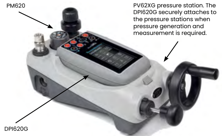
PM620 DPI620G PV62XG pressure station. The DPI620G securely attaches to the pressure stations when pressure generation and measurement is required. Re-rangeable pressure measurement and generation from 25 mbar (10 in H 2 O) to 1,000 bar (15,000 psi)
