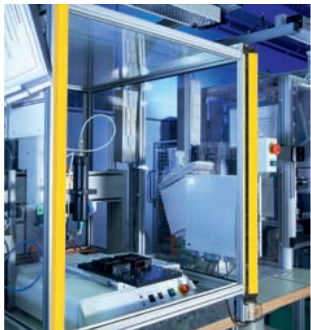
In the past: assembly machine with light curtain
