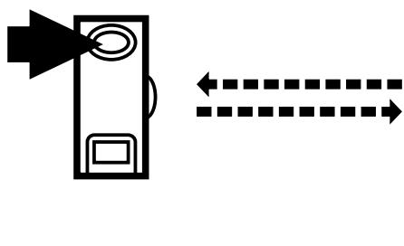
The yellow and green LEDs go out for approx. 1s, after approx. 3s the green LED is on.
