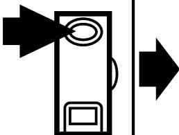
The red LED starts to flash fast after 2s. Then the yellow and green LEDs flash alternately. After 10s all LEDs go off, the output function has changed from light-on mode to dark-on mode (or vice versa).
