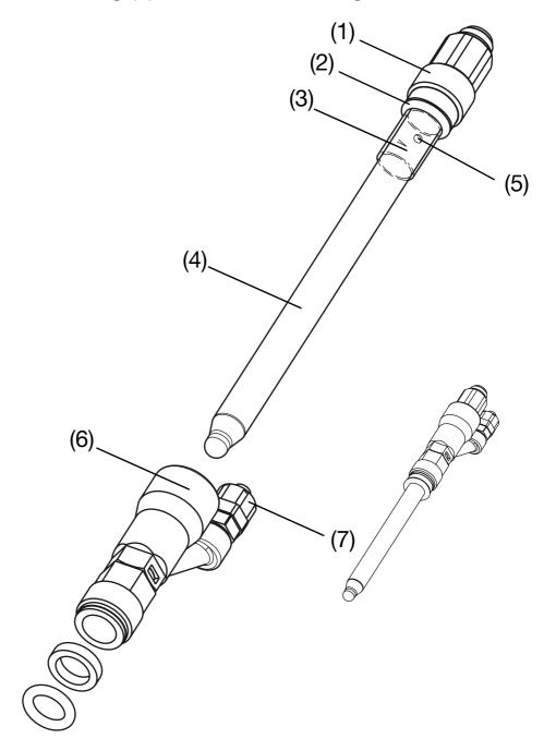
\* Cut the tubular seal open (3) and remove it to expose the filler opening (5).
