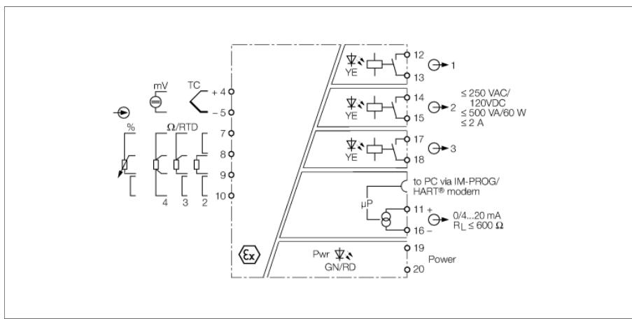
The 1-channel Ex-temperature measuring amplifier IM34-14Ex-CDRi is designed to evaluate the temperature-dependent changes of Ni100/Pt100 resistors and thermocouples types B, E, J, K, L, N, R, S, T and to output them as temperature-linear current signals 0/4...20 mA. Furthermore, resistors, potentiometers or low voltages can be mapped linearly as current signals in a range between -160...+160 mV.
