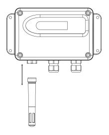
Plug in reference sensor 1/2 and check analogue output
