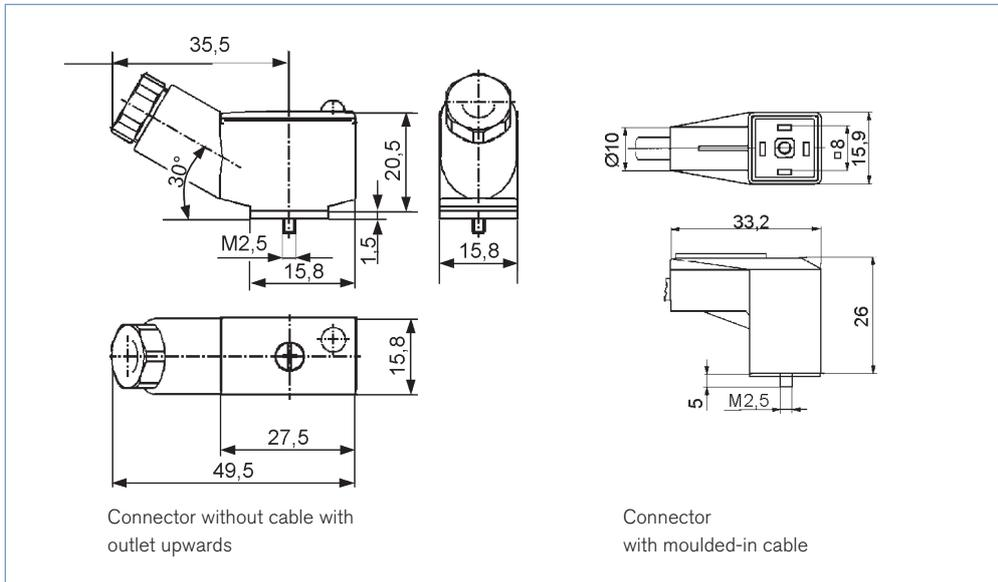
Connector without cable with outlet upwards
