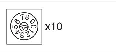
On the upper rotary switch x10, use a small screwdriver to set the tens digit for the address ("3" in the example).
