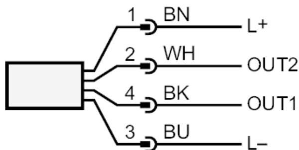
OUT1: switching output or IO-Link
