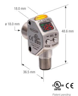
Housing Style Family Output Mode Connector Q3X LD Q8 В **B** = Bipolar **LD** = Laser Diffuse Q8 = 5-pin Integral QD T = 18 mmThreaded 300 mm range QD models require mating cordset **LD50** = Laser Diffuse 50 mm range Barrel with 60 mm BGS\* **LD100** = Laser Diffuse 100 mm range with 120 mm BGS\* \* BGS = Background Suppression
