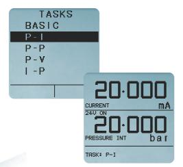
The P-I task configures the DPI 610/615 to simultaneously display the **OUTPUT** pressure and the **INPUT** current. The pressure unit can be chosen to suit the transmitter and a 24V supply is available for loop power. (not IS version).
