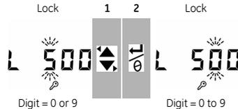
3. To finish the lock code, repeat steps 1 + 2 for each digit. The next time you want to change the menu options, the display shows: L - - - Enter the applicable code. To reset the code to the factory code, you must do a restore operation. Refer to "Maintenance".
