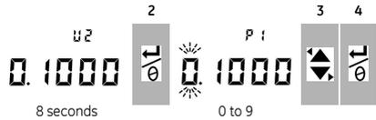
After step 2, the DPI 104 sets Vout to 0.1 V. Correct the value (P1) to the value shown on the voltage calibrator.
