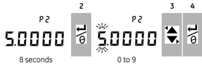
After step 2, the DPI 104 sets Vout to 5.0 V. Correct the value (P2) to the value shown on the voltage calibrator.
