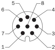
View of M23 male device connector on encoder
