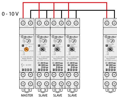
This new system is modular, adaptable to every need and allows control of multiple lamps through a single control device called the "Master Dimmer" Type 15.10.8.230.0010.
