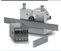
Measuring system with mobile encoder holder, mounted on springs, (with rack and pinion) for an optimum contact pressure and protection of the encoder shaft.
