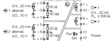
Standard active voltage or current signals are galvanically isolated and transferred via the 2-channel analog signal isolator IM31-22EX-I from the Ex area to the non-Ex area.
