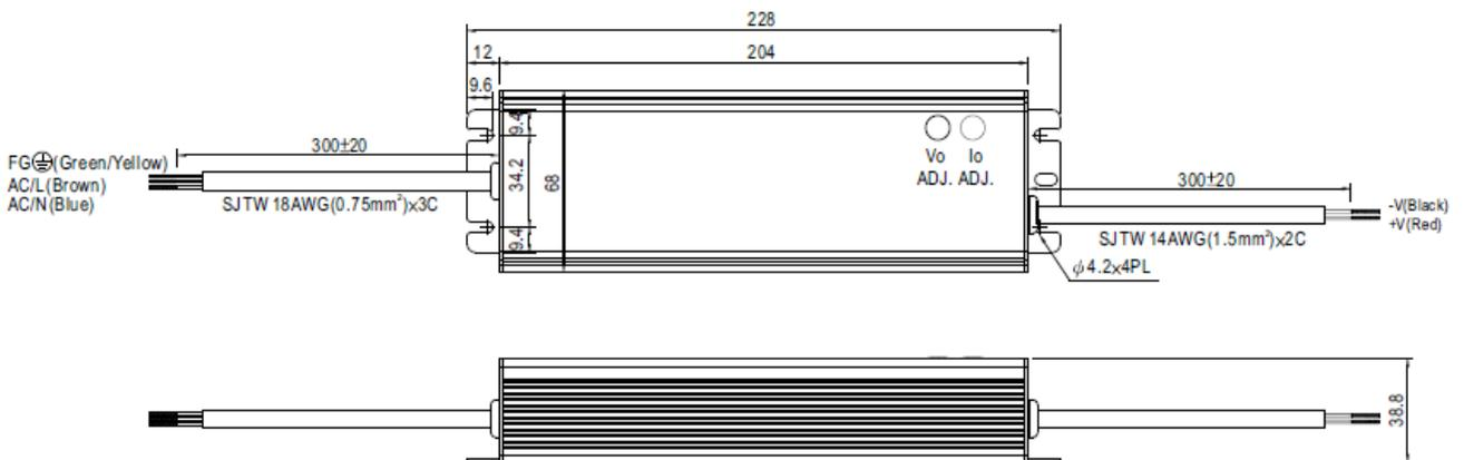
※IP65 rated. Output voltage and constant current level can be adjusted through internal potential meter.
