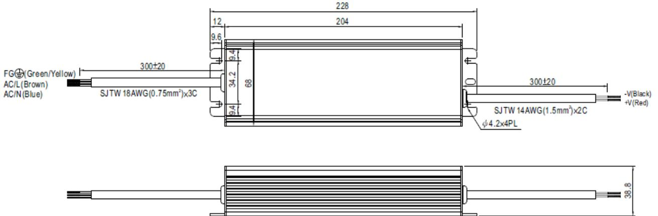
※IP67 rated. Cable for I/O connection.
