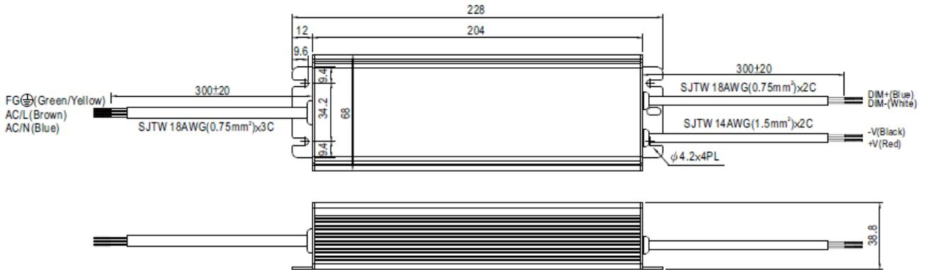
※ IP67 rated. Output constant current level can be adjusted through output cable by connecting a resistor or 1 ~ 10V dc or 10V PWM signal between DIM+ and DIM-.
