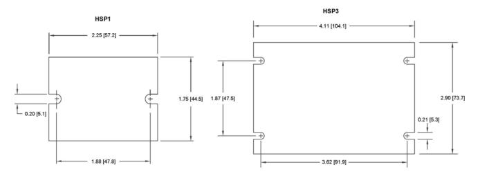
(1) Dispose of separator paper between pads prior to installation of SSR onto heatsink. Installing separator paper with pad may result in relay failure.
