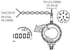
Figure 3: Example configuration: Vout
