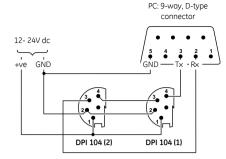
Figure 4: Connections for a DPI 104 network
