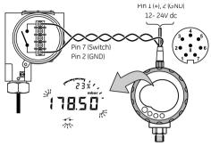
Figure 2: Example configuration - Switch input
