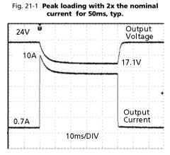
Peak load 10A (resistive load) for 50ms Output voltage dips from 24V to 17.1V.
