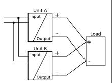
The output voltages of all DC/DC converters shall be adjusted to the same value
