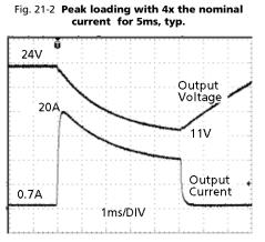
Peak load 20A (resistive load) for 5ms Output voltage dips from 24V to 11V.
